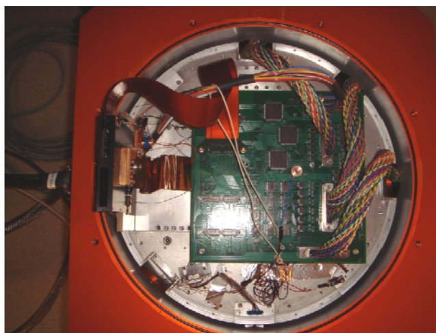
Figure 7. Top view of fully integrated detector electronics system inside the dewar. The detector is mounted on the raft (left) and connected to the cold fanout board (middle).
