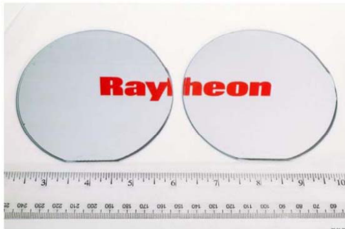
Figure 1: Picture of silicon wafers after having HgCdTe deposited using MBE growth
